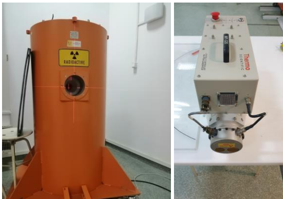
Fig. 2. ^{241}\text{Am}/\text{Be} isotopic neutron source (left) and D-T neutron generator (right) in LWPDiR CLOR
