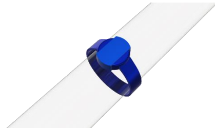
Fig. 2 A ring dosimeter on a finger phantom
