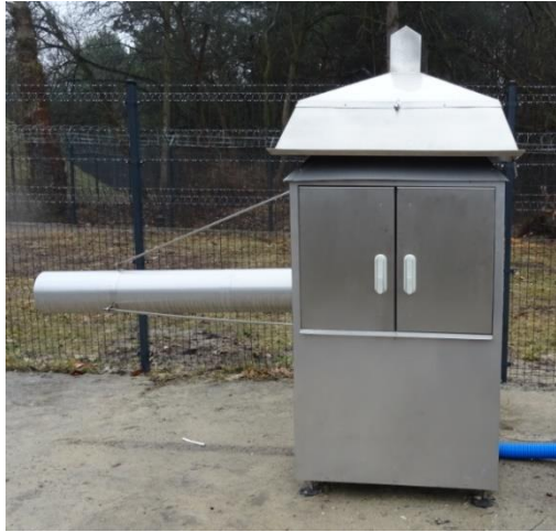
Fig. 1. Housing of the new ASS-500 station
