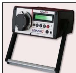
Fig. 2 and 3. Instruments for measuring radon daughters: AlphaGuard (left) and AlphaPm (right)
