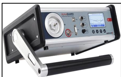
Fig. 2 and 3. Instruments for measuring radon daughters: AlphaGuard (left) and AlphaPm (right)
