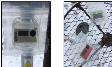
Fig. 2. Exposure of TLD dosimeters
