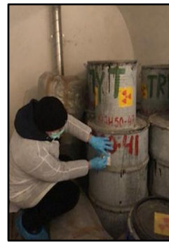
Fig. 3. Taking swabs from tritium waste containers
