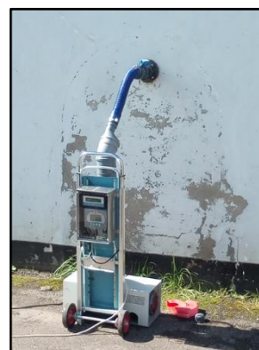
Fig. 6. Station for collecting air aerosols from taps in facilities 2 and 3 of the KSOP in Rózan (CLOR product)
