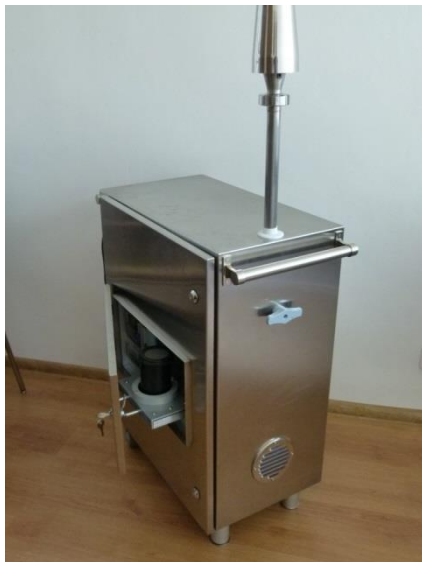
Figure 2. General view of the stand-alone iodine station.
